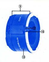
1. Grip the knurled ring (9) of the Macro Spacer in one hand and rotate the coupler ring (10) with the other hand. Align the red line on the aperture ring coupler (12) with the alignment line (16) as shown in the photograph.
