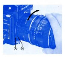
5. When attaching the Macro Spacer combined with the lens to the camera body, attach them after aligning the alignment line (14) with the alignment dot (A) of the camera body, and rotate the lens clockwise until it stops.
