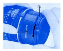
2. The lens can be removed from the Macro Spacer by rotating the Macro Spacer counterclockwise until it stops, while gripping the knurled ring (9) of the Macro Spacer and depressing the lens release button (8).
